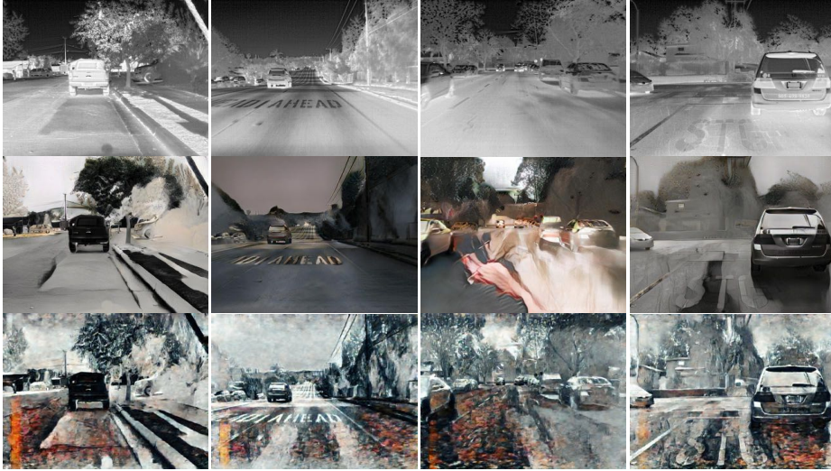
Figure 2.3: Row 1 : Thermal images from FLIR ADAS[1] dataset; Row 2 : Translations generated using UNIT[4]; Row 3 : Translations generated using CycleGAN[5].
